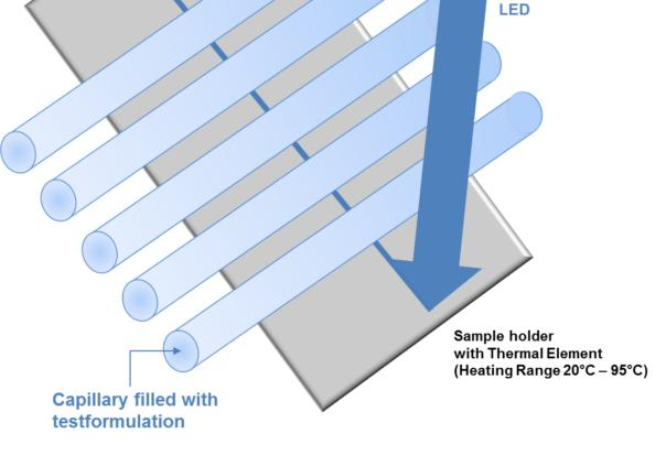
Schematic representation of NanoDSF setup: It is an advanced Differential Scanning Fluorimetry technology based on the detection of changes in chemical and thermal stability of proteins (modified according to Prometheus NT.48 product information).
